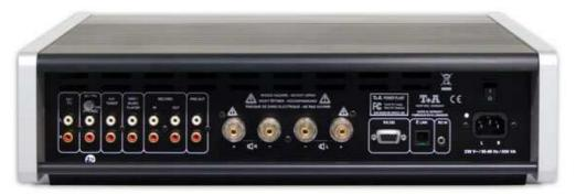
The amplifier features five high-quality inputs which are selected using gold-contact relays, and one of them can be fitted with the internal R-series PHE MM or PHE MC module to provide a phono input (earth terminal fitted as standard). REC OUT and PRE OUT are also present. The solid metal loudspeaker terminals are gold-plated and devoid of ferro-
